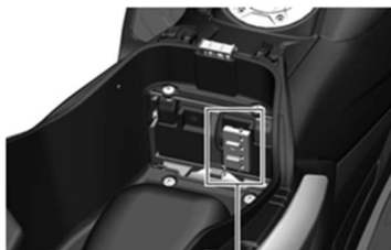
The main fuse box
