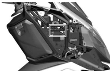
Auxiliary fuse box
